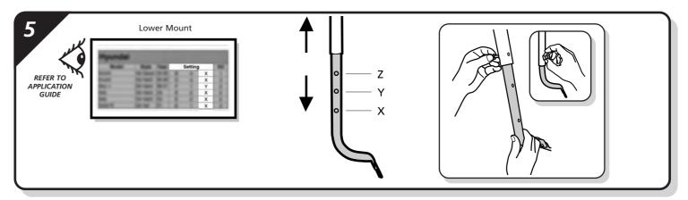
Refer to the enclosed application list to find the correct position for the thumb screw nuts to the inside of the carrier frame. extendible feet X, Y or Z. Insert the bolts from the outside faces, fit the
